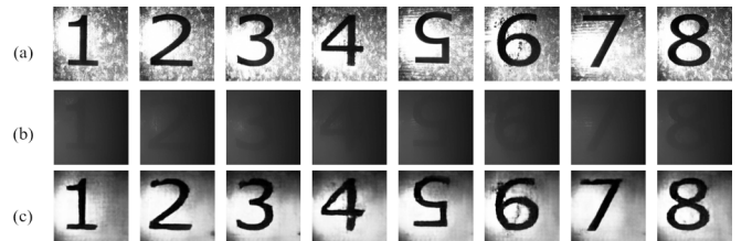
Fig. 4. The test results of untrained digital targets. (a) Ground truth; (b) The scattering images ( S_0 ); (c) Reconstructed images.
