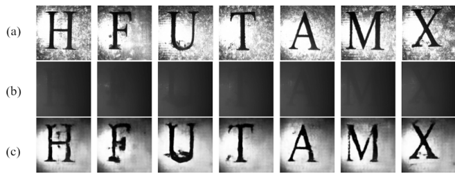
Fig. 5. The test results of untrained alphabetical targets. (a) Ground truth; (b) The scattering images ( S_0 ); (c) Reconstructed images.
